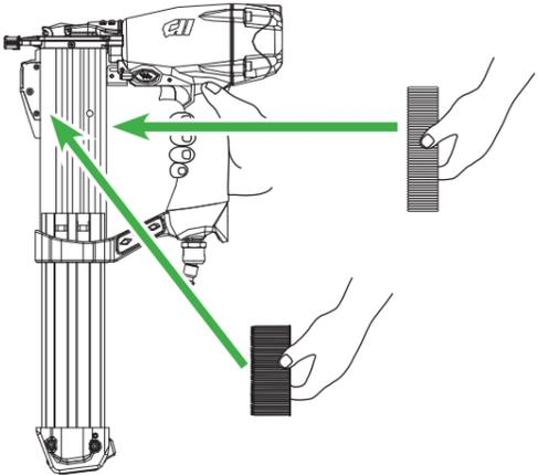
**Load** nails with points all the way into the groove. Load staples with crown straddling the rail.
