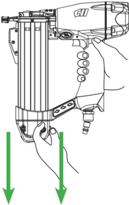
**Press** magazine latch button and pull magazine open.
