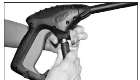
Figure 5 - Attach high pressure hose to gun
