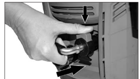
Figure 8 - Attach high pressure hose
