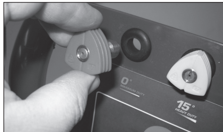
Figure 11 - Insert spray tips into the holder
