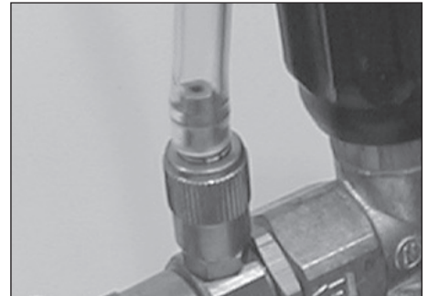
Figure 10 - Attach suction tube to barb fitting
