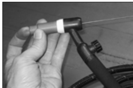
Figure 4 - Tungsten should stick out 3/16"
