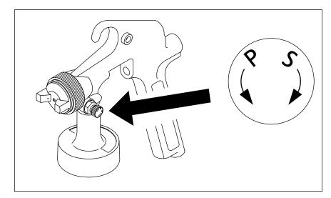
To change from Siphon Feed to Pressure Feed mode, turn the knob shown above from 'S' to 'P' until finger tight.
