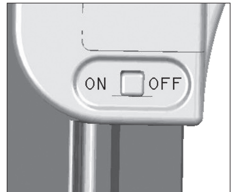
Figure 18 - Electronic ON/OFF Switch
