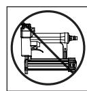
**DANGER** Do not touch the trigger unless driving fasteners. Never attach air line to tool or carry tool while touching the trigger. The tool could eject a fastener which will result in death or serious personal injury. Also actuate the trigger guard to the safe position when not in use.
